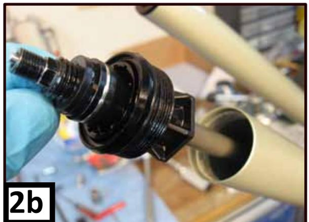
4. Using the Mattoc Cassette Tool and a torque wrench (a socket will fit over the Cassette Tool, shown in picture) tighten the compression rod end cap down to:
