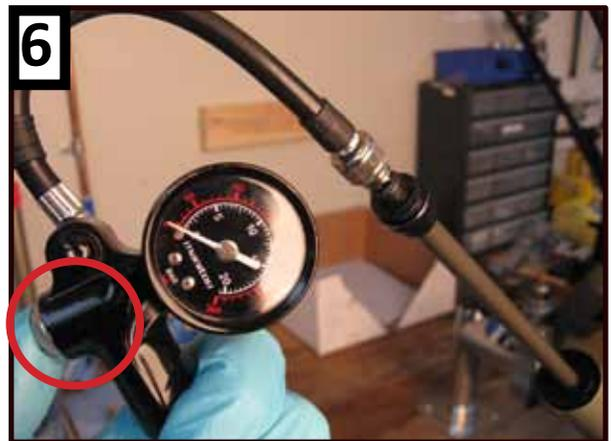
**⚠️ WARNING** Air pressure must be released prior to disassembly of the fork. Failure to properly and fully release air pressure could result in serious injury or death.
