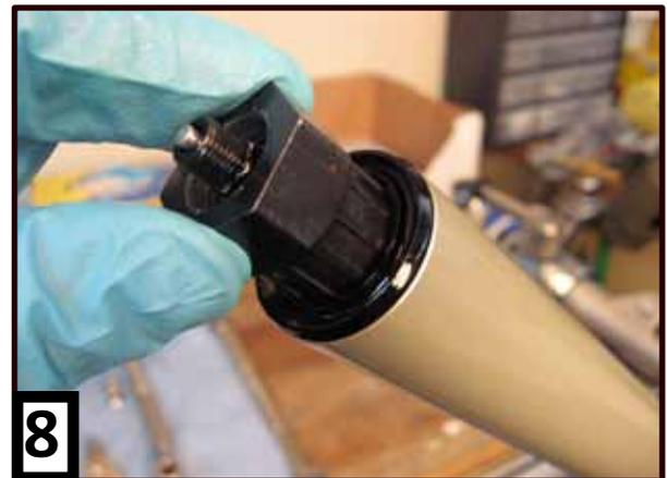
9. Using an adjustable wrench or similar tool, turn the cassette tool counter clockwise to remove compression rod assembly from fork stanchion.
