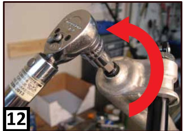
13. Using the Mattoc 11mm Thin Wall socket (part number 172-31130) and torque wrench, tighten the compression rod into the casting by turning it **counter-clockwise**. Tighten to 30-40 in lbs. [3.5-4.5 Nm].
