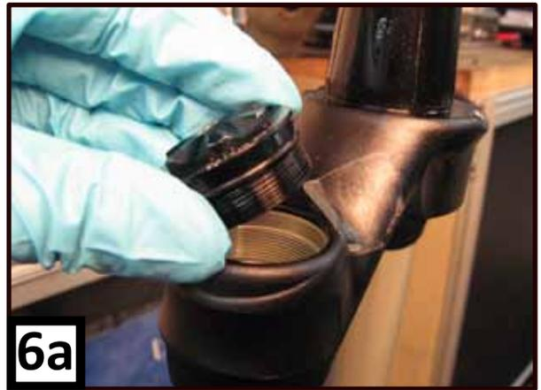
6. Install Air Cap using the Mattoc Flat Ground 24mm Socket (Part Number 172-31131) and torque wrench. Tighten cap to 60-80 in lbs. [6.8-9.0 Nm].
