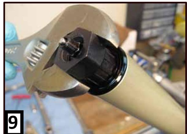
10. Remove compression rod assembly from fork.
