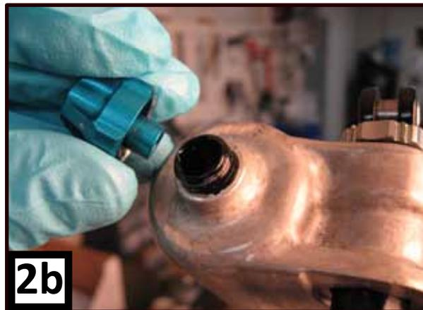
3. Insert an 8mm Allen wrench into the end of the rebound damper rod. Turn wrench **clockwise** until damper rod can be pushed into fork casting.
