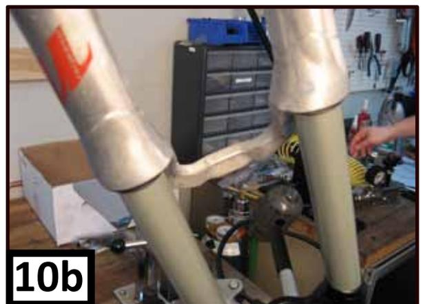
11. Insert 15cc's of Manitou Semi-bath oil into each side of the casting.
