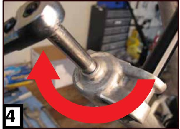
5. Remove casting from the fork. It is recommended that this be done over a drain pan as there is semi-bath oil in the lower legs that will be released when casting is removed.
