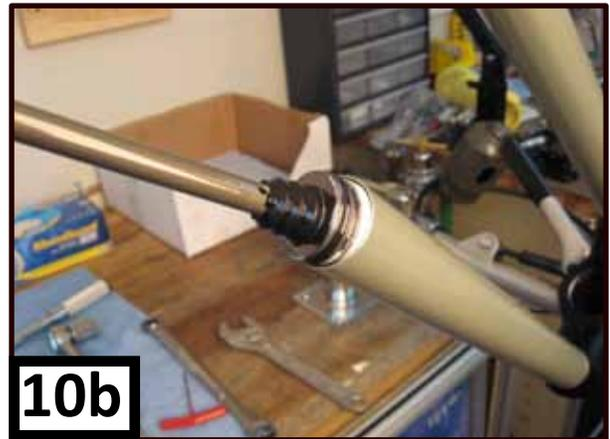
11. Using the Matroc 24mm Flat Ground Socket (part number 172-31131), slowly remove the air cap from the fork.
