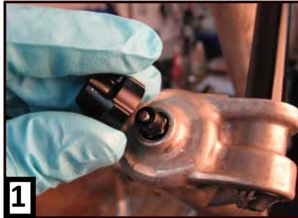
2. Using a 2mm Allen wrench, remove the rebound damper knob.
