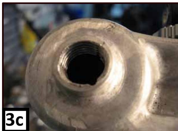
4. Using the Matroc 11mm Thin Wall Socket (Part Number: 172-31130), turn the compression rod **clockwise** until compression rod is disengaged from the casting threads.
