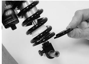
Note: If the spring will not clear the mounting hardware, the hardware must be removed and re-installed after the new spring is installed. Care should be taken when removing or installing the mounting hardware as to not damage the DU bushing or eye.
