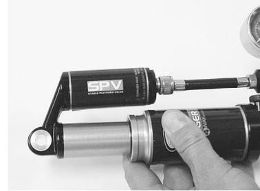
shock pump to fine tune your air pressure. The hiss you hear when unscrewing the pump is only the air left in the pump itself and not from the shock! This does not affect your pressure setting in the shock. Likewise, when you install the pump, the shock will fill the pump and reduces the registered pressure
